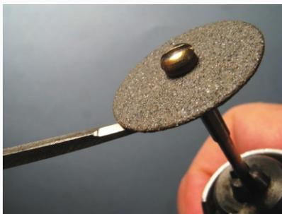
After sawing patterns there's always a little cleanup to do, and the smaller cutouts can be a challenge. Needle files (7-8 inches) can get into the larger areas, and escapement files (4 inches) can get into some of the corners.
